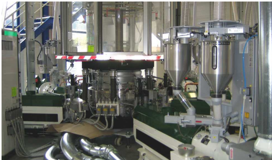
7-layer Co-Extrusion line with gravimetric dosing units
