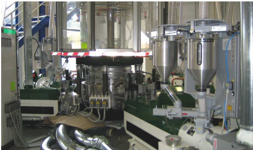
7- layer Co-Extrusion line with gravimetric dosing units
