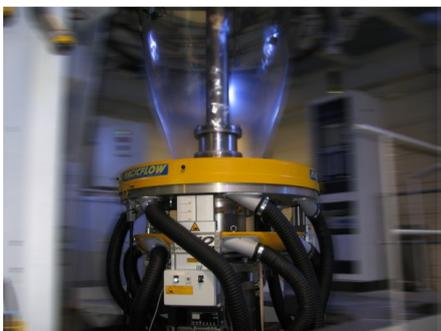
Control of the cooling air volume – increased or decreased volumes of segmented cooling air regulated in relationship the thick or thin points around the bubble influencing the thickness of the film below the frost line. This procedure is almost energy neutral as each cooling air path is volumetrically isolated with each other (the number of which varies with the air ring diameter), as one area of the bubble requires less cooling air another sector requires more balancing
