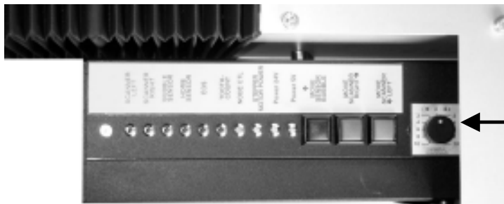
Potentiometer to adjust contact pressure
