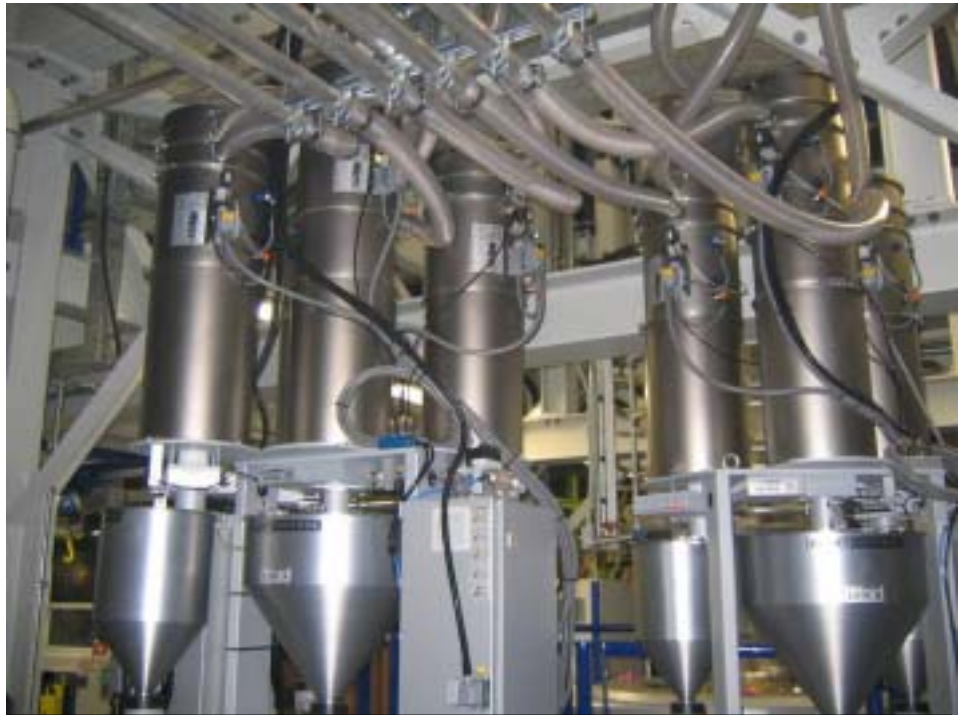
PCH Loaders and Ballast Hoppers mounted directly on to the weighing hopper.
