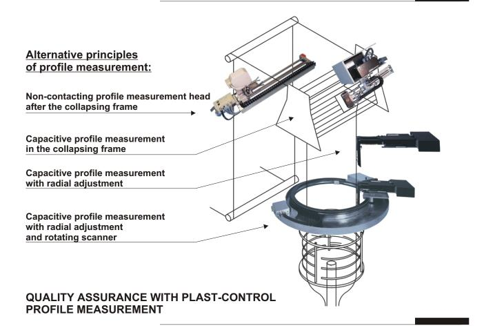
The ASC PRO-FIL is a blown film gauge profile measurement system designed to measure film while in production. The system is capable of measuring and displaying the gauge profile of up to four lines on a single computer and monitor. The standard system includes computer, software, monitor and one gauge, gauges for additional lines are optional.
